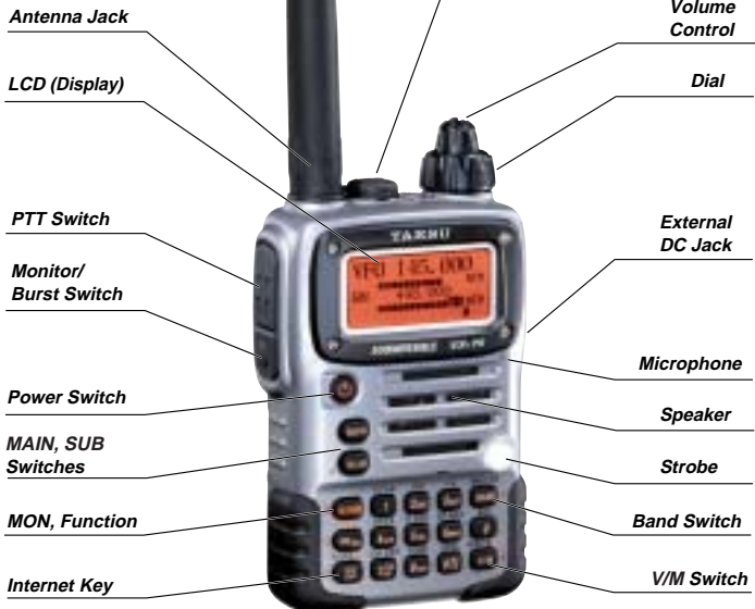
Innovative Multi-section Antenna! When operating on 144 and 430 MHz, use the bottom section of the supplied antenna. For operation on 50 MHz, simply screw on the antenna extension element and you're ready for DX action!
